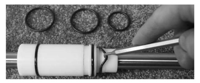
16. Replace O-ring on piston (Kit Item 'I'), piston seal (Kit Item 'G'), and wear ring (Kit Item 'C'). Note the piston seal sits, with the open end towards the bottom of the pump. Place bushing on rod. Do not forget to replace upper bumper (Kit Item 'K') Tighten Piston housing and Piston nut.
