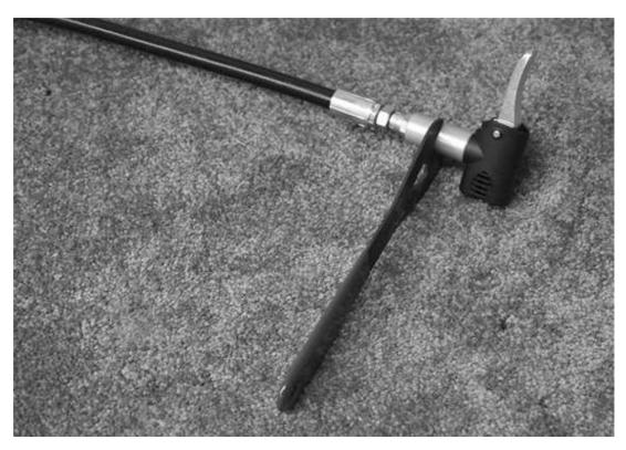
2. Place 16mm Cone Wrench in the slots of the aluminum hose adapter (attached to Air Chuck)
