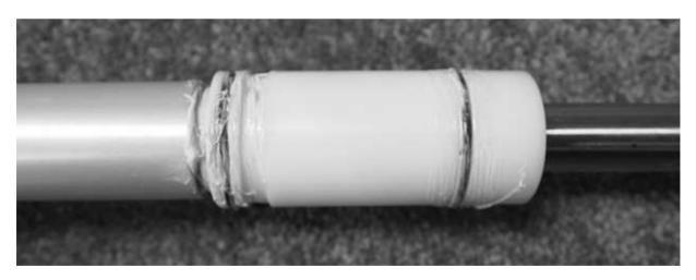
21. Re-grease o-ring on Foot Valve. Replace Foot Valve into bottom of Pump Tube.
