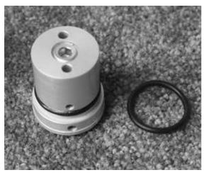
11. Remove the bottom piston nut using adjustable wrench and 16mm wrench. Remove piston seal (Kit item 'G').
