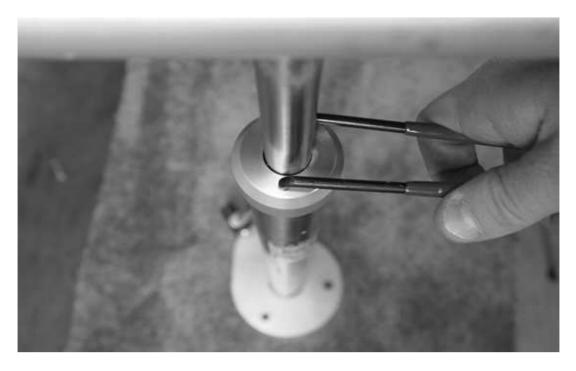
26. Test the pump by inflating a bike tire. Leave the pump connected to the pressurized bike tire and listen for leaks.
