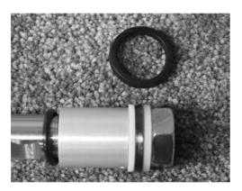
17. Re-grease o-rings on Bushing. Place a thin layer of grease below the bushing on the Pump Rod.
