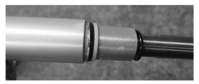
20. Press Pump cylinder on to Bushing until it is snug on the last o-ring and it feels like it has "clicked" into place.
