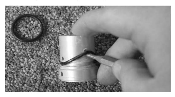
8. To replace the Check Ball, use a screwdriver and a 4.5mm (3/16") Allen wrench to remove the plug from the Foot Valve. The screwdriver should fit in the bottom holes. Turn the brass plug counterclockwise to remove.
