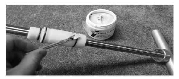
18. Grease top of Pump Cylinder (Bottom Bumper should still be in the bottom of the Pump Tube).
