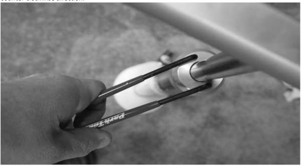
2. Remove the contents of the pump by standing on the pump housing flange and pulling the handle out. Due to the o-rings on the bushing, this may be tight.
