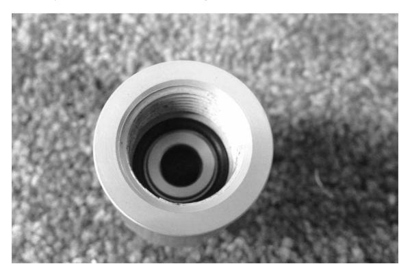
14. Remove rod wiper seal using a pliers. Be careful not to damage plastic. Replace wiper seal (Kit Item 'F'). Be careful not to damage the seal.
