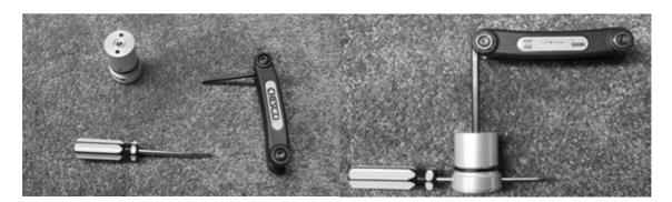
9. When the brass plug is free, remove the Check Ball and clear the Foot Valve of any obstructions. Replace the check ball (kit Item 'E').
