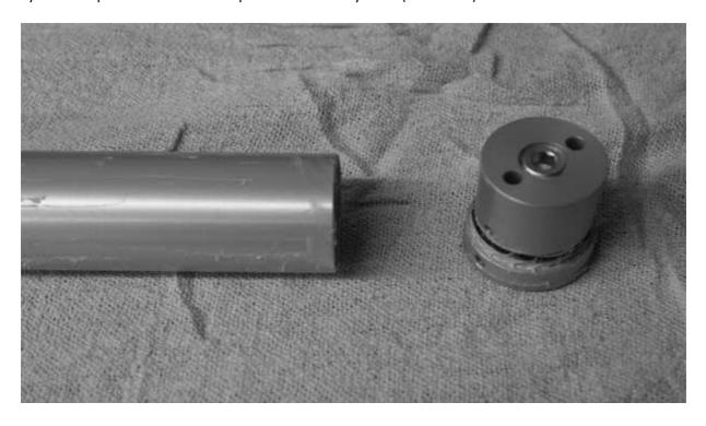
7. Remove o-ring from Foot Valve and replace with O-ring (Kit Item 'H').
