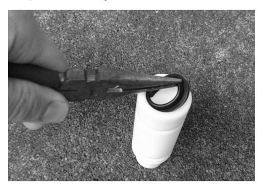
15. Remove o-rings that are to be replaced on the bushing. Replace with new o-rings (Kit Item 'H' and 'M'). Take care not to damage the o-rings on any material edges they may have to go over.
