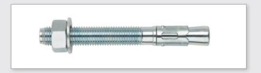
The recommended minimum diameter of the rod axis is 12 mm and it can be 14 or 16 mm in special cases. The minimum length required for anchoring in concrete should be 10 cm (5 cm within + 5 cm piece under floor) depending on the type and pavement condition. In any case, it is recommended to always consult the manufacturer's data sheet.
