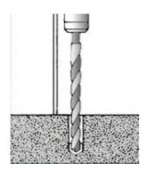
7. Before proceeding with installation, the hole must be cleaned of all concrete dust to ensure proper fastening. Use a wire brush, a vacuum or compressed air to clean out the hole completely.
