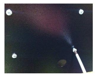
4. Thread in vibration absorbing feet into the compressor's base.
