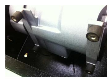
5. Install smaller screws into the vibration absorbing feet. Do not over tighten screws!
