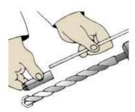
6. Before starting to drill the hole, it is important that eye and ear protection are used. Make sure the hammer drill is in the hammer mode and start drilling your hole. Continue drilling until the tape on the bit or the drill gauge meets the base material- this means that the required depth has been reached.
