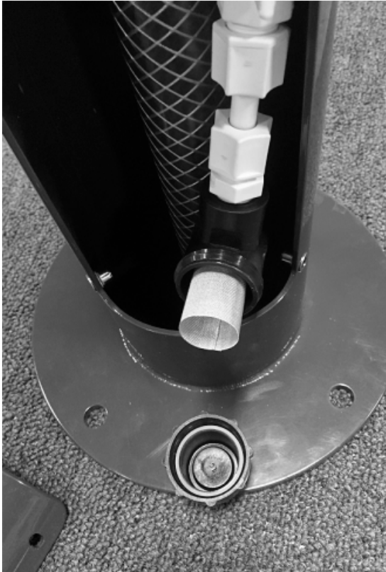
Figure 13: Inlet strainer cap removed for cleaning.
